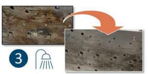
Flush / wash off the mold surface with a degreaser.
